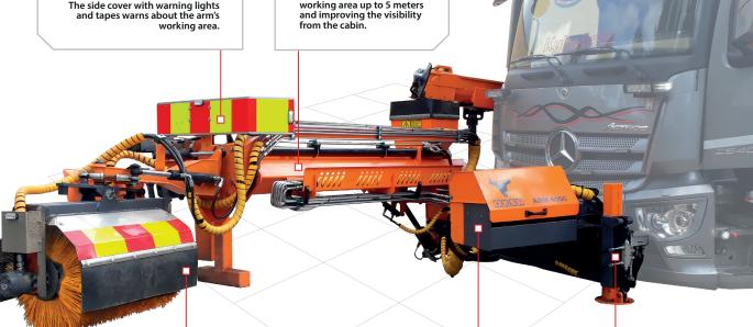
With arm's brush tool you clean up any dirt from pothole in no time.
