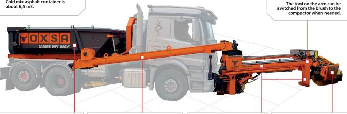
Asphalt container tilts forward, tipping the mix asphalt onto the auger at the side of the truck.
