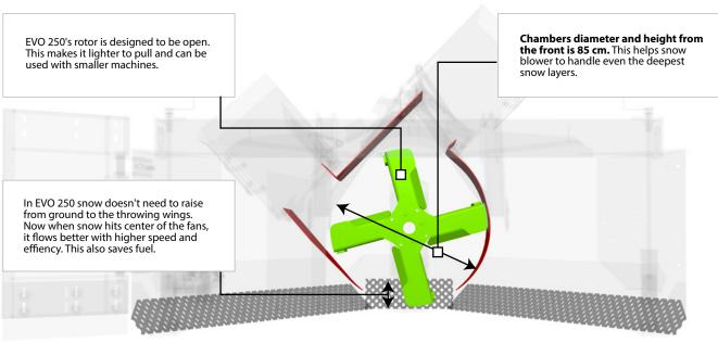
EVO 250's advantages to more tradional models are; lighter to pull (15 - 20 % fuel saving), higher work speed, easier maintenance and cleaner clearing track from its structural design.
