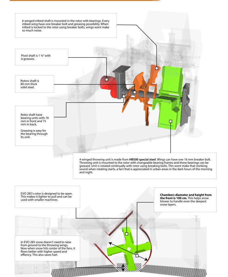
OXSA EVO 285's advantages to more tradional models are; lighter to pull (15 - 20 % fuel saving), higher work speed, easier maintenance and cleaner clearing track from its structural design.
