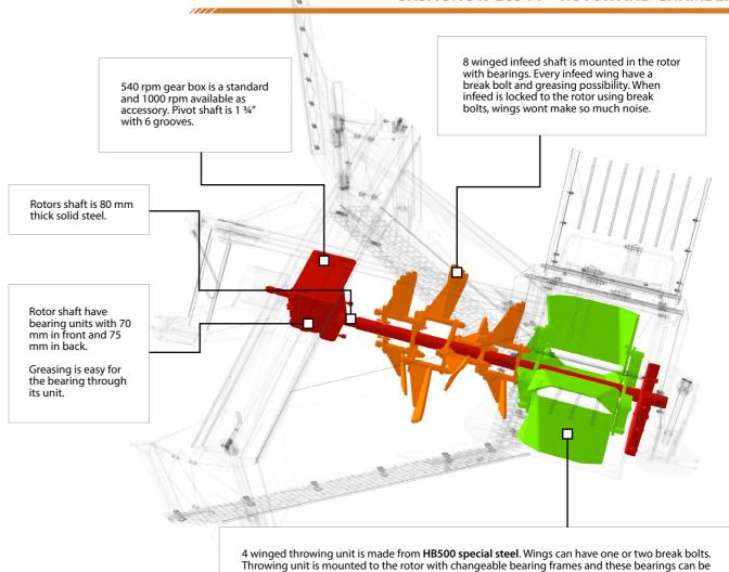
Chambers diameter and height from the front is 100 cm. This helps snow blower to handle even the deepest snow layers.
